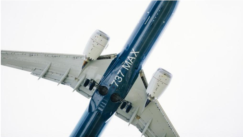
Here is a picture of the 737 Max Engine forward placement in relationship to the Center of Gravity:
