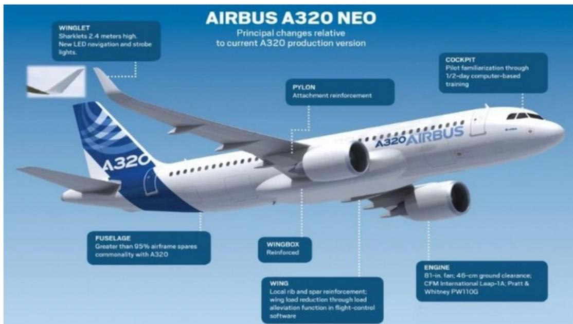
According to the following document, the A320-200 has 24 inches of clearance from the bottom of the engines to the ground and the A320-NEO has 18 inches of clearance. [https://www.airbus.com/content/dam/corporate-topics/publications/backgrounders/techdata/aircraft\\_characteristics/Airbus-Commercial-Aircraft-AC-A320.pdf](https://www.airbus.com/content/dam/corporate-topics/publications/backgrounders/techdata/aircraft_characteristics/Airbus-Commercial-Aircraft-AC-A320.pdf)
